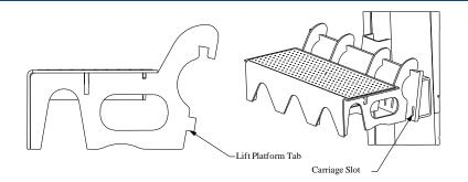
11. Align the lift units so that they will be as shown in the figure below when the Forklift Adapter is fully assembled. Ensure that they are directly across from each other. If the optional 3 Wheel Adapter (shown) is used, it must be centered between the outside ramps.
