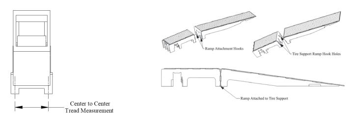
15. If the 3 wheel adapter is to be used, align the tabs on the Lateral Support Bar with the ramps and slide it back as far as possible. All three ramps must be captured by the Lateral Support Bar.
