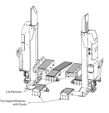
14. Install the ramps as shown in the figure below. Ensure that the Ramp Attachment Hooks are fully inserted into the Tire Support Ramp Hook Holes and the ramps are able to contact the floor.
