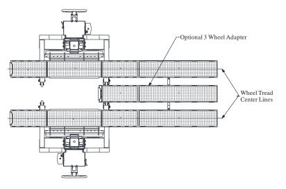
12. Adjust the distance between lift units until the center lines of the ramps and tire supports will be the same as the center to center tread measurement on the forklift to be lifted as shown in the figure below. After adjusting, lower the base of each lift unit to the ground. Ensure the lifts and adapters are properly aligned. If the 3 Wheel Adapter is to be used, this distance may need to be adjusted slightly to accommodate the Lateral Support Bar.
