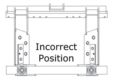
Secure the end lift adapters to the lift units with the locking pin brackets. Insert and rotate the pins so that they point toward the outside of the lift unit's carriage after installation, as shown below.
