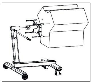
Fig. 4: Mounting engine to stand
