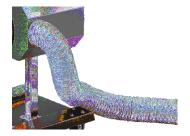
Adjust the height of the EV-1 to place the suction mouthpiece as close as possible to the exhaust pipe. Lock the wheels of the unit. Turn on the EV-1 and then start the engine.
