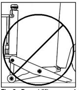
Fig. 9: Do not lift on rounded surface
