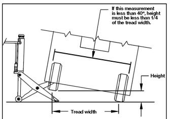
Fig. 4: Lifting height versus forklift width
