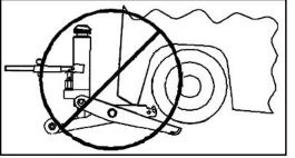
Fig. 8: Only use the notch/lift pad to lift forklift
