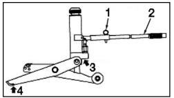
Fig. 2: Lock handle in place to wheel and/or lift jack
