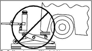
Fig. 7: Never increase lifting height
