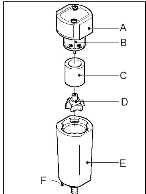
**Note:** A periodic check of the automatic drains is necessary to ensure the membrane life. To verify float is functioning correctly, open the filter bowl by turning one quarter turn counter-clockwise. Inspect for water or oil, an inactive float will be submerged, an active float will not. If float is found to be inactive follow cleaning procedure below or if necessary replace with part number 026-80386-00.
