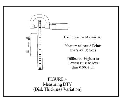
reading labeled Point 2. Rotate the rotor another 90 degrees and record the reading labeled Point 3, and then again another 90 degrees labeled Point 4. The difference between Point 1 and 3 will be the Maximum Run Out. Disc Flatness will be the <u>highest</u> difference between: Points 1 and 2: Points 2 and 3: Points 3 and 4: <u>or</u> Points 1 and 4.
