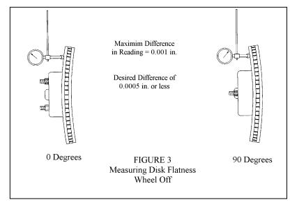
To insure the highest degree of precision, it may be advisable to check Disc Flatness nearer to the outside diameter of the rotor. (See Figure 3)
