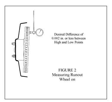
Instead of the rotor being a series of perfect rings, it is a series of rings that become increasingly deformed as the rings become larger, again like the brim of a hat. A similar result would occur if the rings were twisted. In either case, Disc Flatness can be measured with the same dial indicator as used to check run out. Except, to check Disc Flatness, the rotor is rotated 90 degrees.
