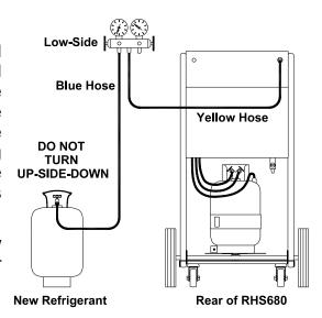
DO NOT TURN THE CYLINDER OF NEW REFRIGERANT UP-SIDE-DOWN AS LIQUID REFRIGERANT WILL BE INTRODUCED INTO THE RHS680. COMPRESSOR DAMAGE COULD RESULT WHICH VOIDS THE WARRANTY.
