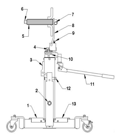
Fig. 1: Component identification
