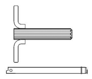
Fig. 11: 1.75" diameter spline adapter
