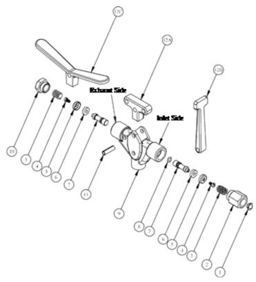
Fig. 7: Air valve exploded view
