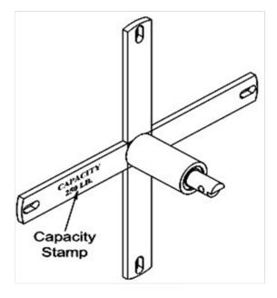
Fig. 10: Flywheel adapter - Rear View
