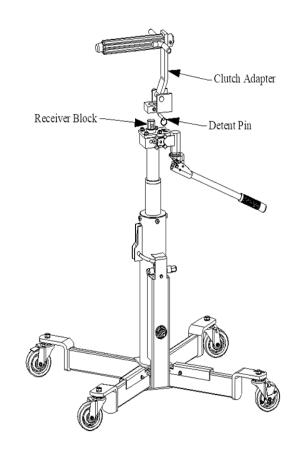
Fig. 8: 2" Spline Adapter
