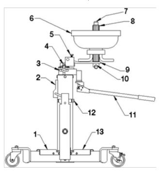
Fig. 4: Loading/unloading clutch from jack
