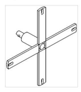
Fig. 9: Flywheel adapter - Front View
