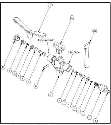
Fig. 7: Air valve exploded view
