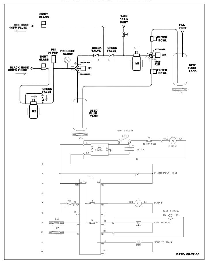
ATX-2 PLUS BOOSTMACHINE ELEC & FLOW (2008)
