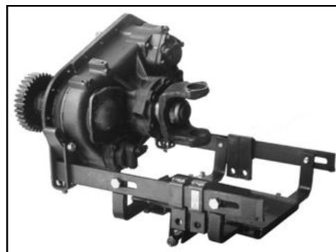
Fig. 24: Adjusting brackets to eliminate interference
