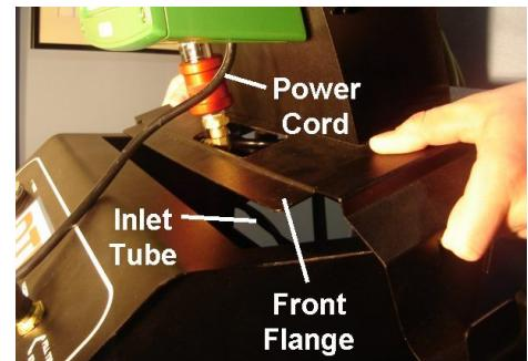
Route power cord through access hole and out through the rear of the NTF-15 cabinet. Check that grommet is inserted in bracket where hose to the Valve is routed.
