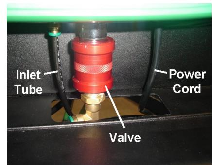
Disconnect coiled hose. Remove fitting from the right side of NTF-15 and install it with the New Tee supplied.
