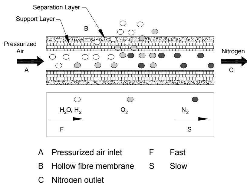
Ambient air contains nitrogen (78.1%), oxygen (20.9%), argon (1%), carbon dioxide, water vapor and traces of other inert gasses. Pressurized air (A) is fed through the hollow fiber membrane (B). The various air components diffuse through the wall of the membrane.
